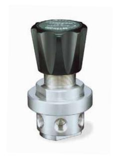
TESCOM 44-2900 Series backpressure regulator is designed to be compact, extremely sensitive and for industrial gases with flows up to 20 SCFM / 566 SLPM. The convoluted Stainless Steel diaphragm provides excellent sensitivity and repeatability; metal-to-metal diaphragm seal minimizes the potential for leakage.
